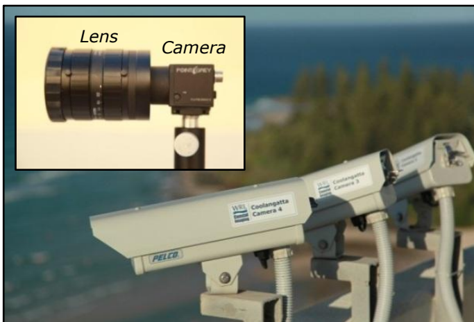
Left – Coastal Imaging Cameras in Position (Inset: Lens and Camera). Right - Schematic of an Entire Coastal Imaging System
