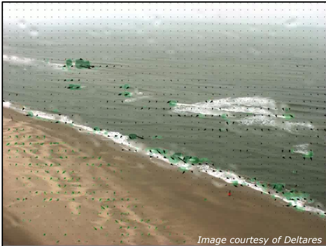
Left: Argus image showing optically sensed surface currents Right: Fourier transform analysis of time stack image to yield directional wave spectra
